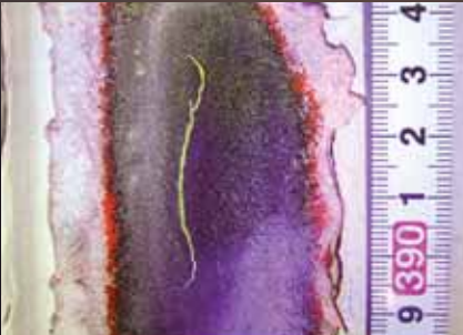
疲労き裂の検出
